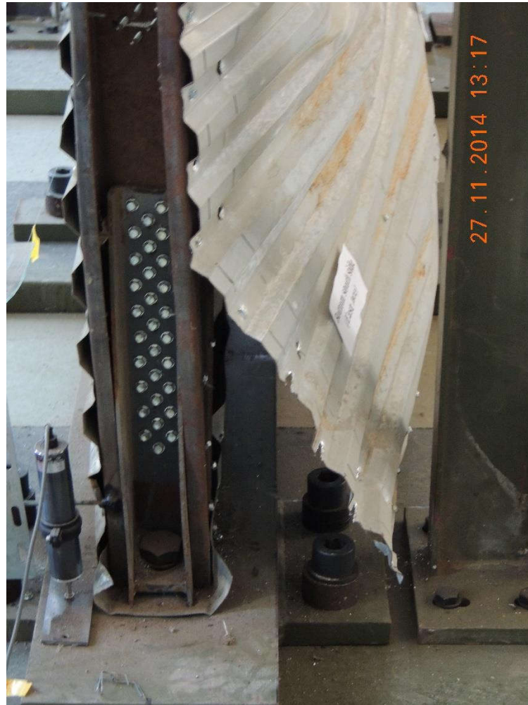
Fig. 1.14. Screws pull-through and tear out-bearing [24].
