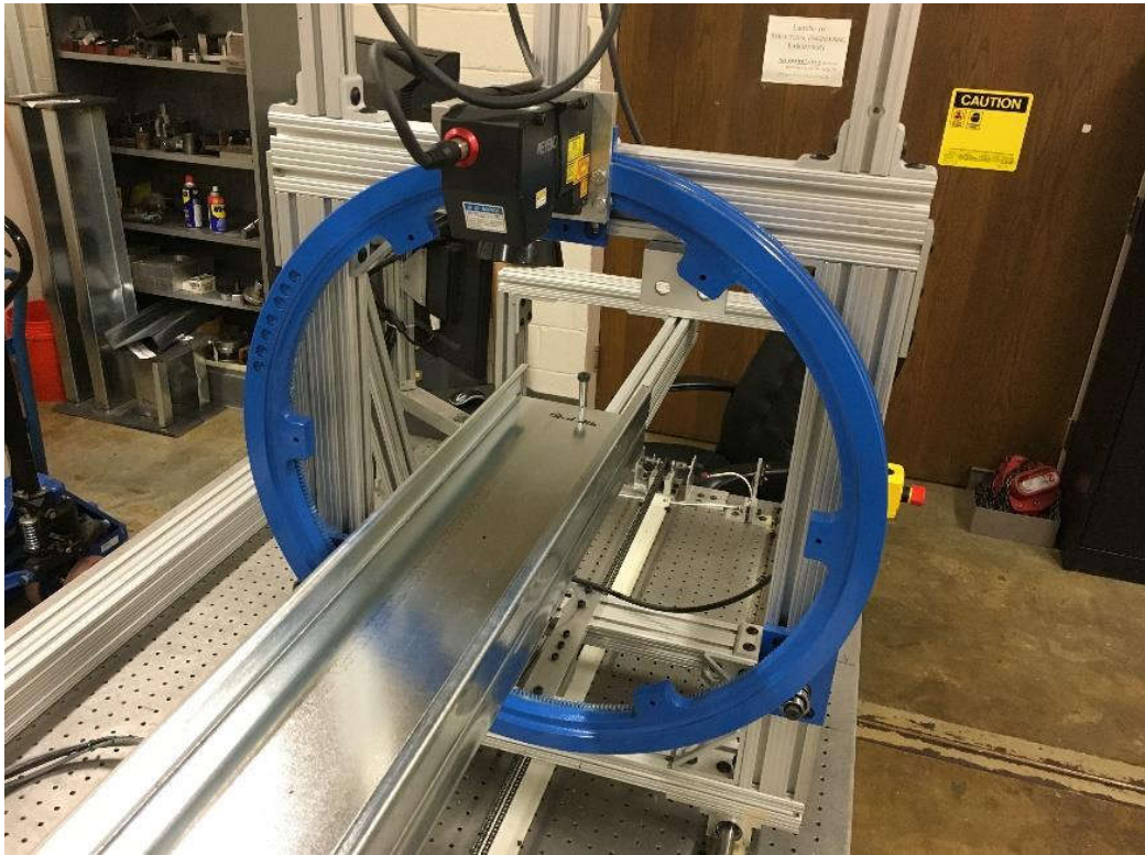
Fig. 6.6. Laser scanner setup with built-up specimen installed.
