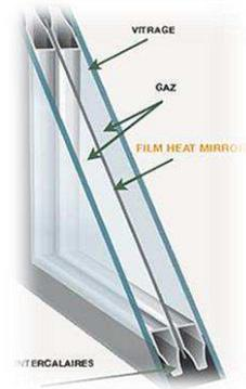
Figure III-68: detail double vitrage
