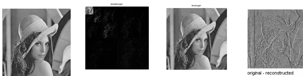
Figure 5.17 : Lena image and its level 3 DWT, reconstructed image, and the difference between original and reconstructed one.
