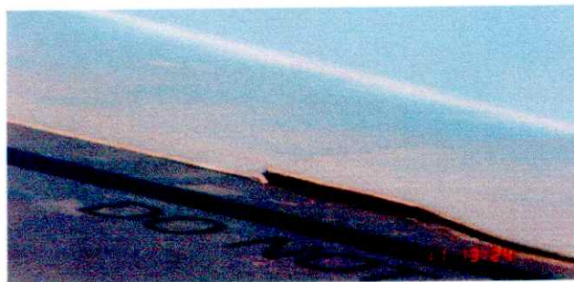
Figure B2 - Example of misrigged slat
