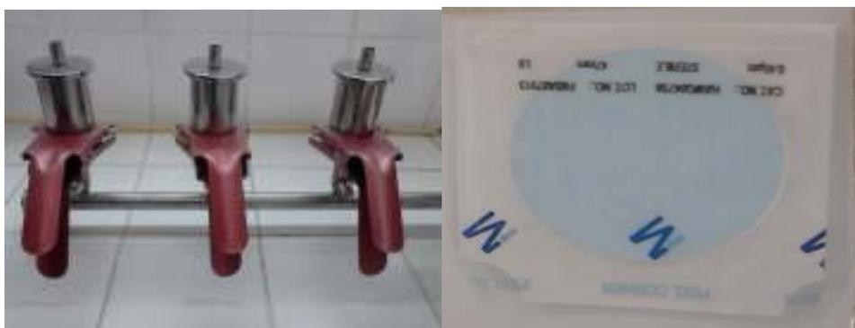
**Figure 03.** Ramps filtrante **Figure 04.** Membranes filtrante
