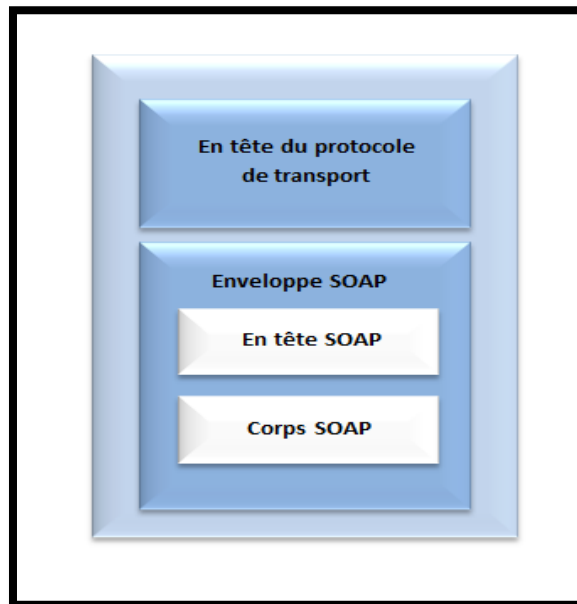
Figure I-8: Structure de message SOAP. [25]
