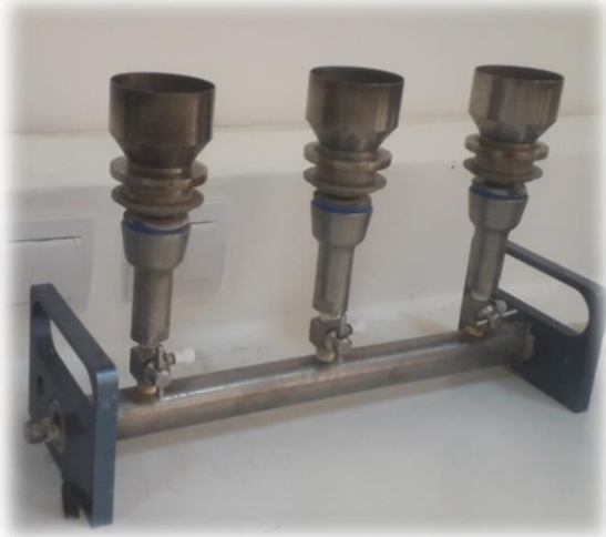
Figure 25: Rampe de filtration.
