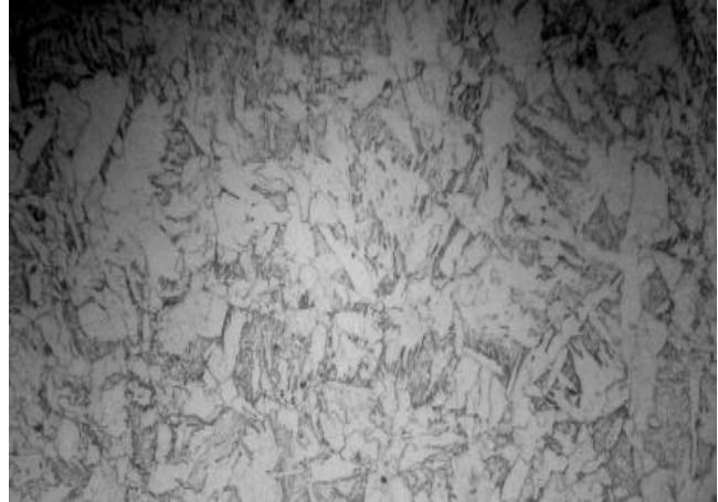
Fig.15 Structure Ferrite polygonale + perlite + ferrite aciculaire
