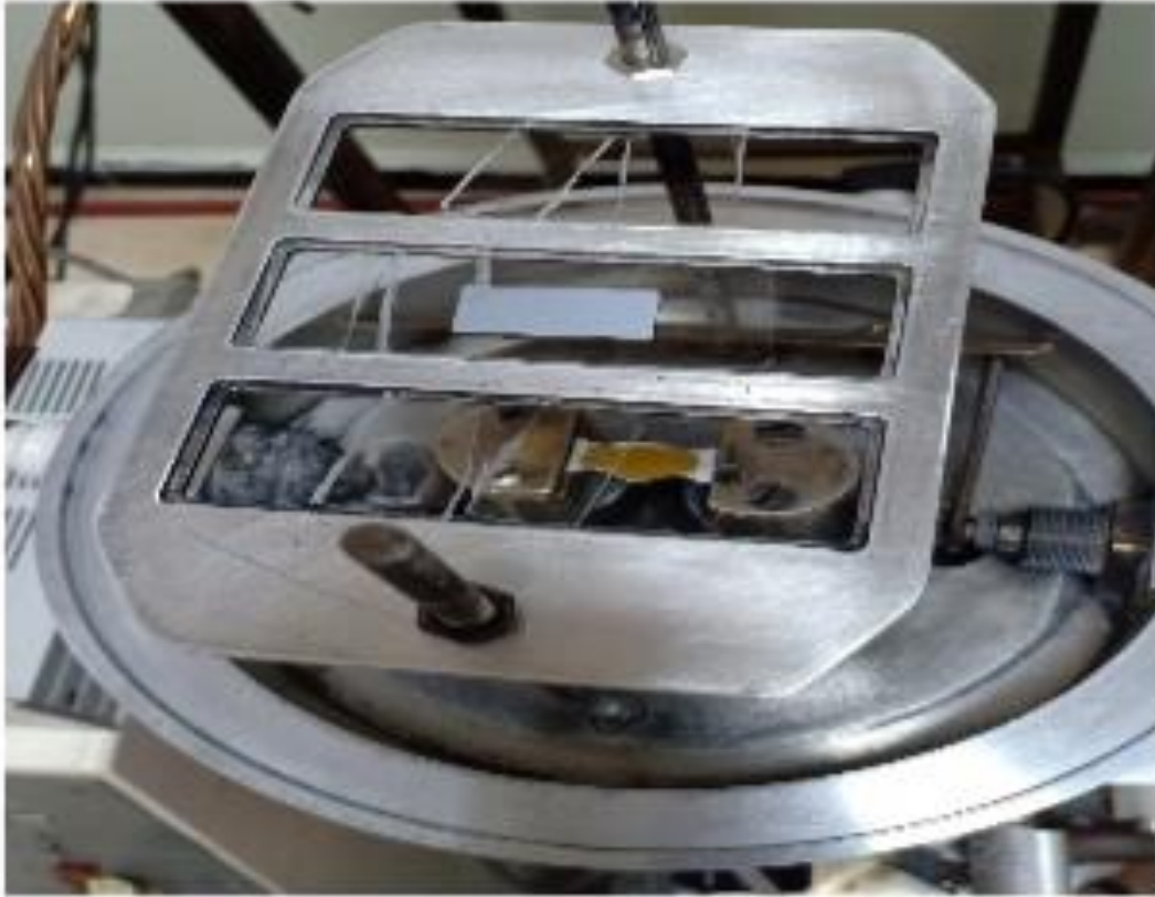
Figure2.7 : The deposition method of VO x thin layers in a vacuum chamber(CDTA).
