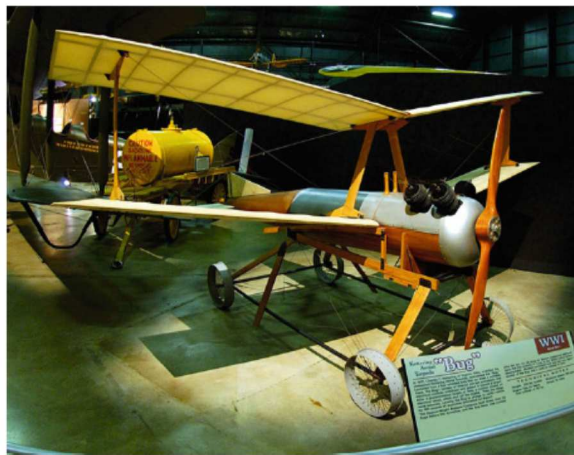
Figure I. 2 The USAF Liberty Eagle Aerial Torpedo, also known as the Kettering Bug after
