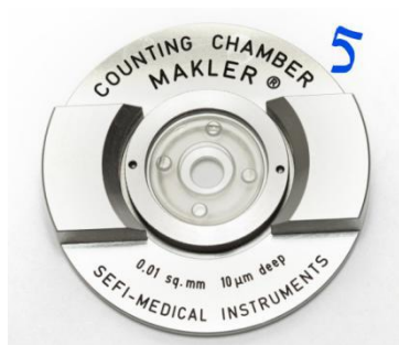
Figure 27 : La chambre Makler® (Microptics, 2018)
