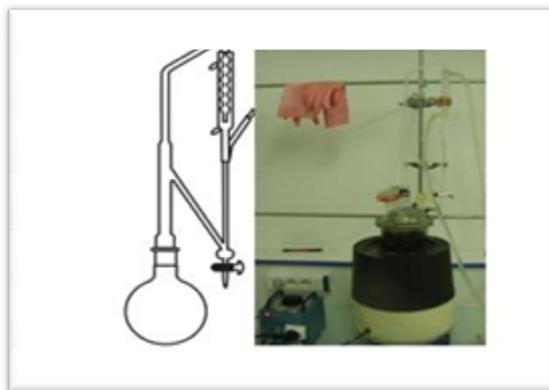
**Figure 10 : Montage d'hydro-distillation (Sutour,2010)**
