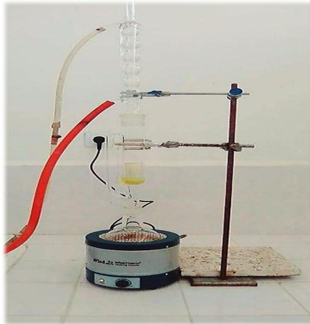
Figure 26 : Appareillage Soxhlet.
