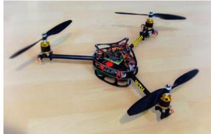
Figure 1.5 : Drone tri-rotor.
