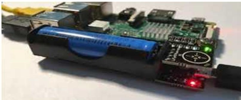
**Figure II.19:** Le LiFePO4wered.
