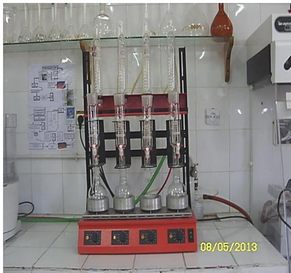
Figure 15 ♦ Appareil soxhlet
