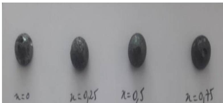
Figure III.2. Lingots Cu_2ZnSn(Se_{1-x}S_x)_4 obtenus.
