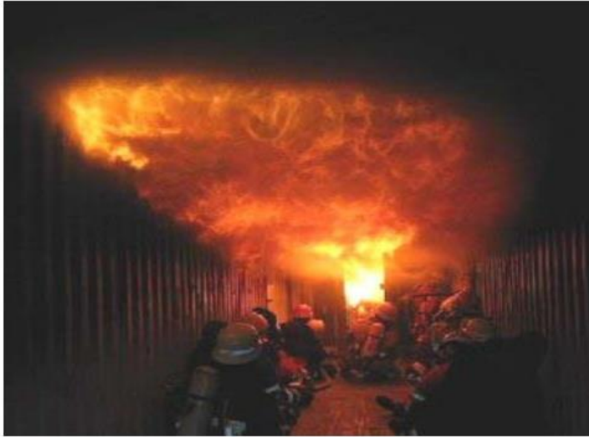
FigureI.10: A simulation of a rollover in a German training container [7].
