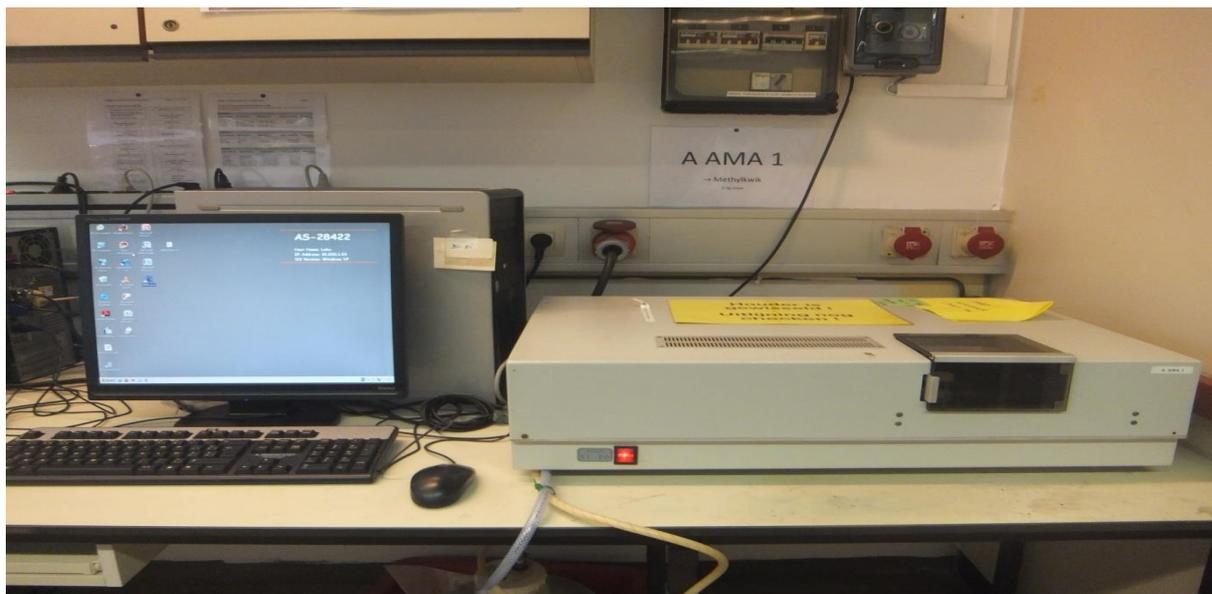
**Figure 5.4 :** Analyseur de Methylmercure ( AMA-1 Methylmercury analyzer).
