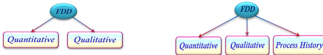
Figure III.6 - Classification of FM methods into: (a: left) qualitative and quantitative methods. (b: right) qualitative, quantitative and process history-based methods.
