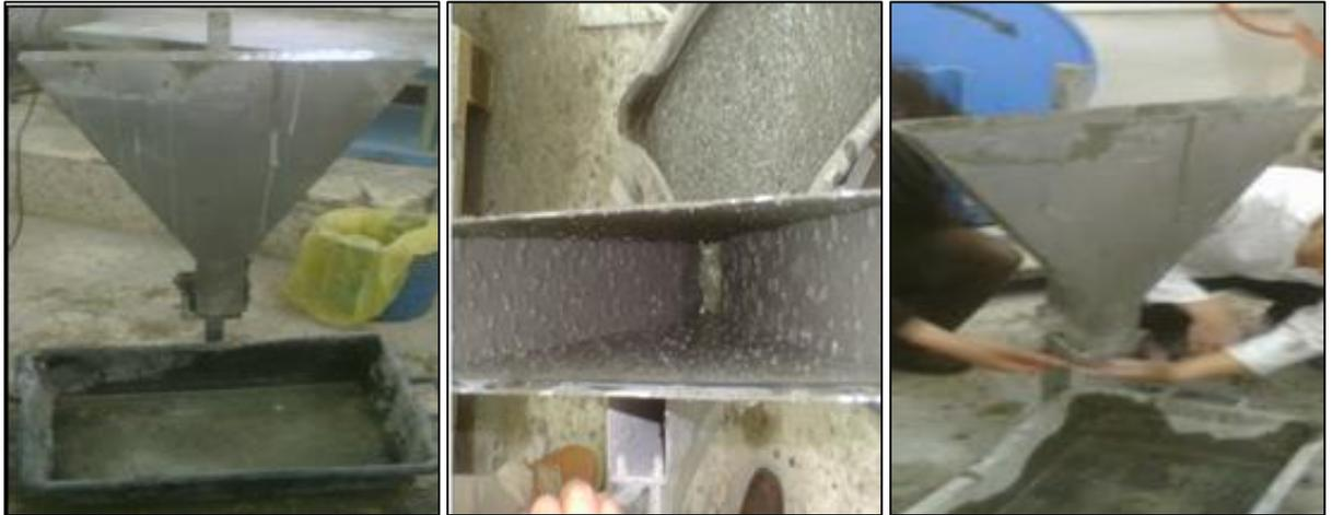
Figure 3. 12: Essai V-funnel.
