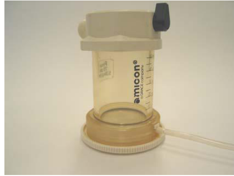
Figure 4.5 : Cellule Amicon de filtration frontale (Amicon – Millipore)
