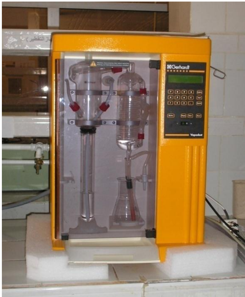
Figure 8.3: Appareil de Kjeldhal (LCI) Photo personnelle
