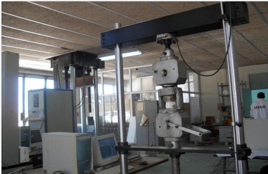
Figure 2.15 :MACHINE D'ESSAI DE COMPRESSION
