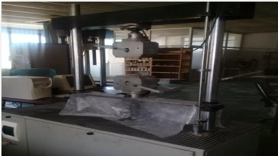
Figure 2.13 : MACHINE D'ESSAI DE FLEXION
