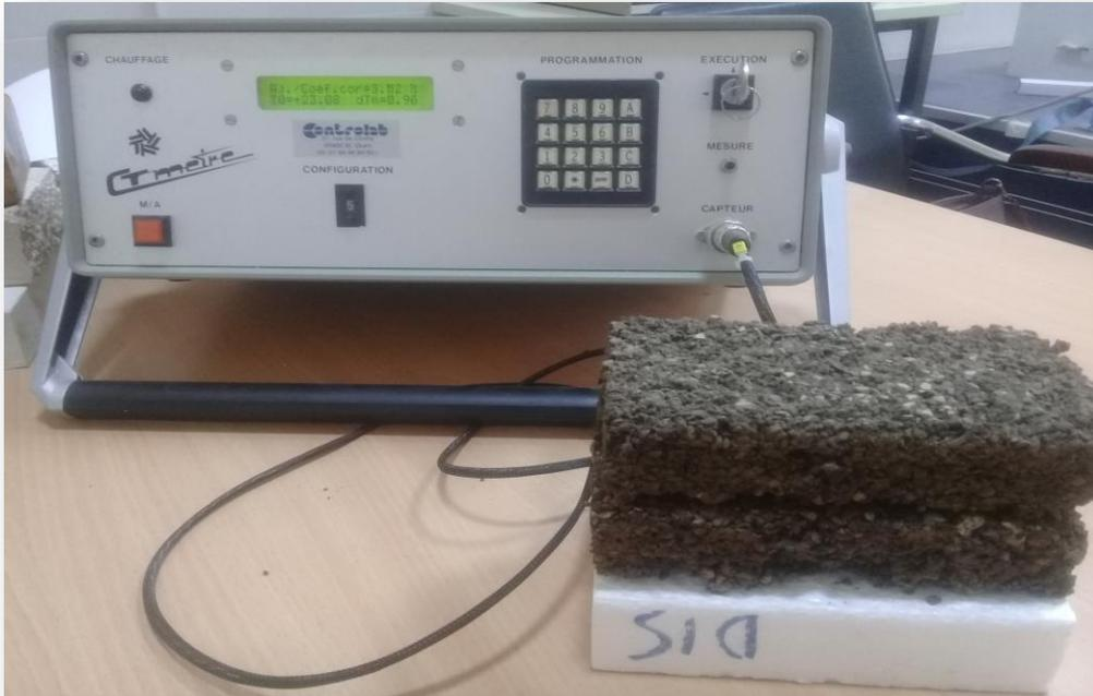
Figure 2.26 : MESURE DE LA CONDUCTIVITÉ AVEC LA MÉTHODE DU FIL CHAUD
