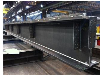
Figure 176: poutre PRS source:Belhocine, 2016
