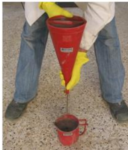
Figure 3.9 : Cône de Marsh.
