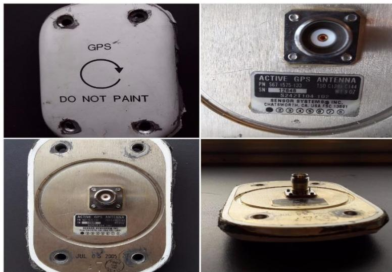
Figure I-20 Active GPS antenna S67-1575-133
