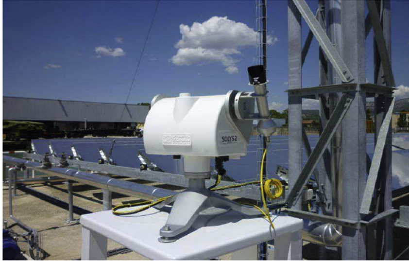
Fig. 3. Pyrheliometre with sun tracker for DNI measurement.
