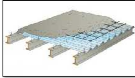
Figure 118 : plancher collaborant. Source : Benattallah et Ramdani, copyright.
