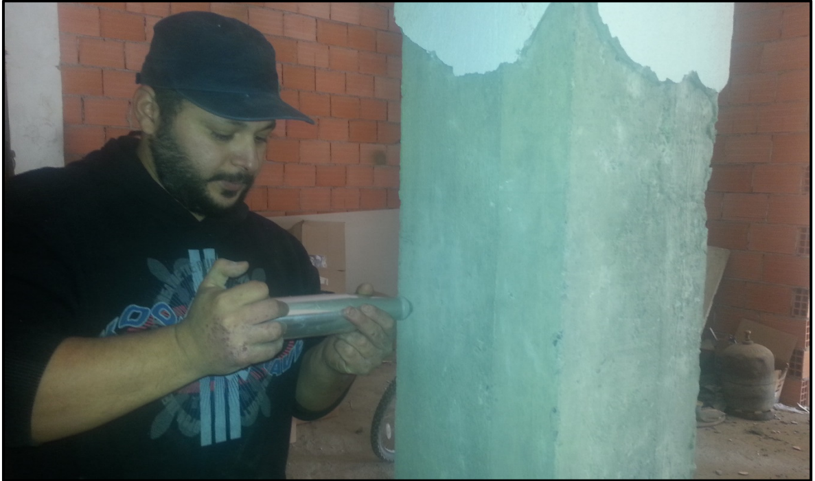
Figure II.29: Measuring the compressive strength of concrete using the concrete hammer test.
