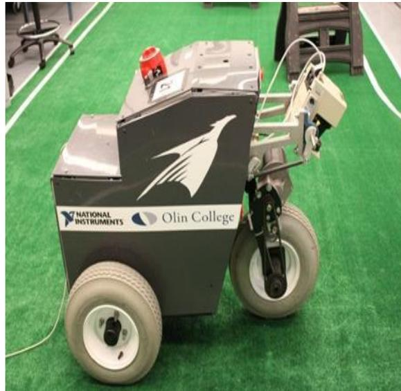
Figure 2.8 Robot de type tricycle
