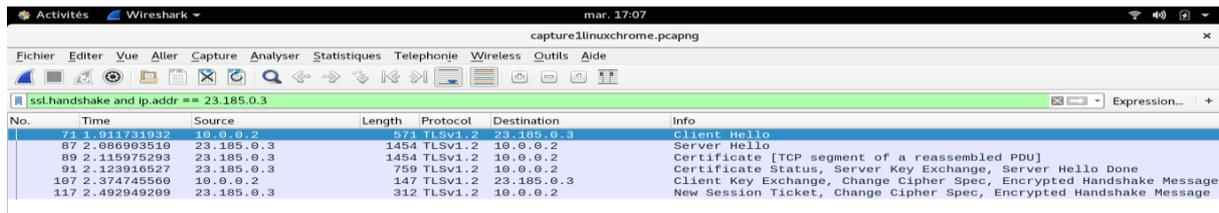
The image shows a Wireshark capture of an SSL handshake. The filter is 'ssl.handshake and ip.addr == 23.185.0.3'. The packet list shows several TLSv1.2 packets. The packet details pane shows the 'Client Hello' packet (No. 71) with the following information:
