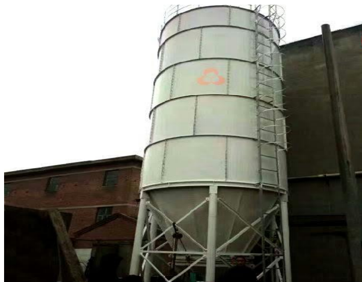
Figure 2.2 : Silo de stockage.
