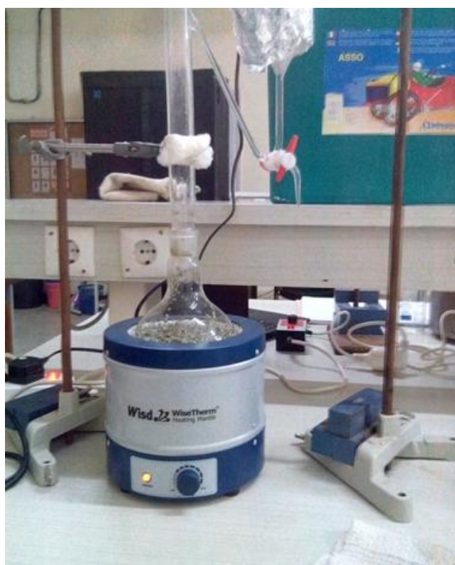
Figure 7: Dispositif d'hydrodistillation type Clevenger (originale, 2018)
