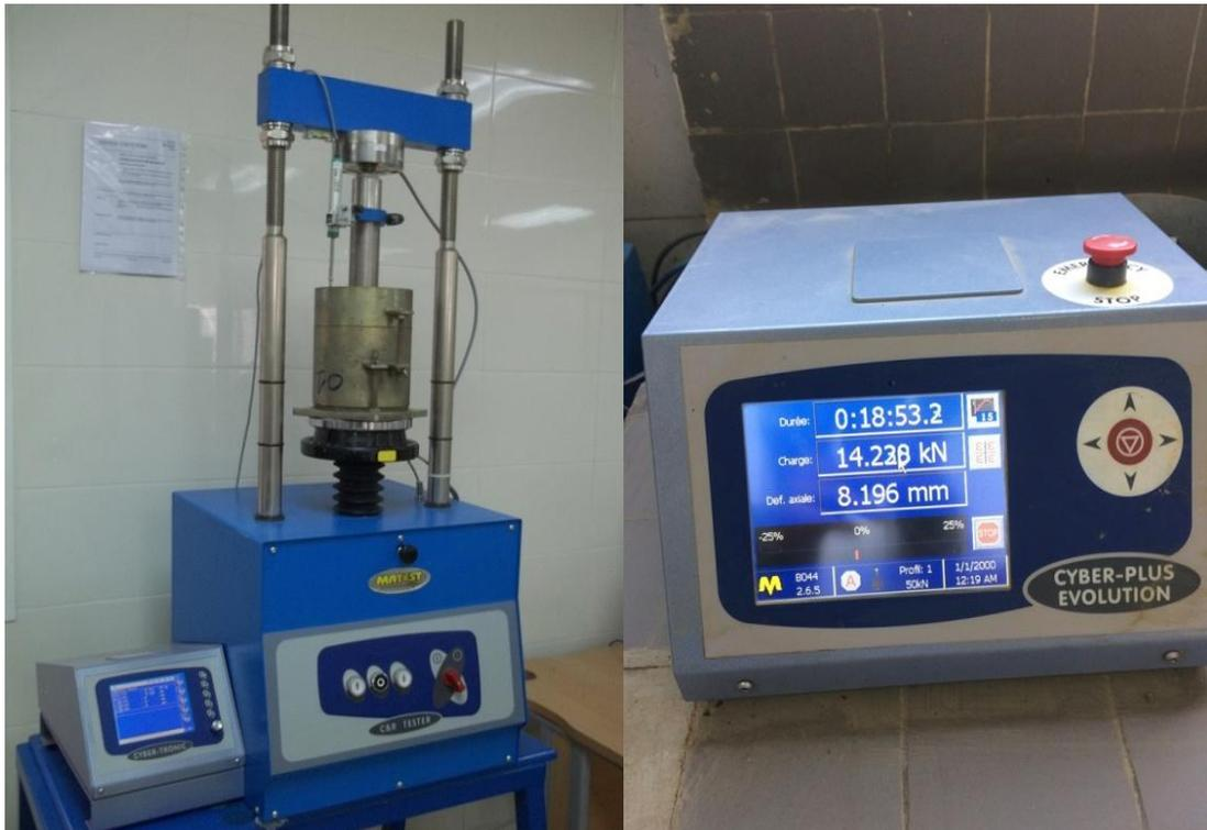
**Figure IV.14 : Essai CBR, (LCTP, Alger).**
