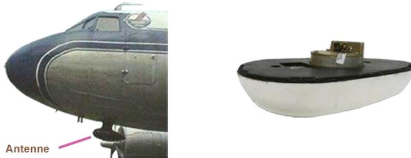
Figure I.14 : Antenne ADF
