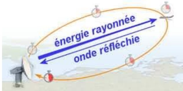
Figure I.2: Principe du radar
