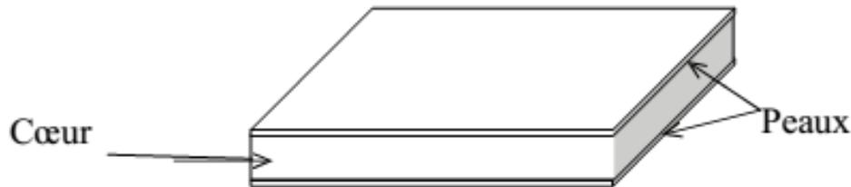
Figure I- 11 : Composite sandwich.
