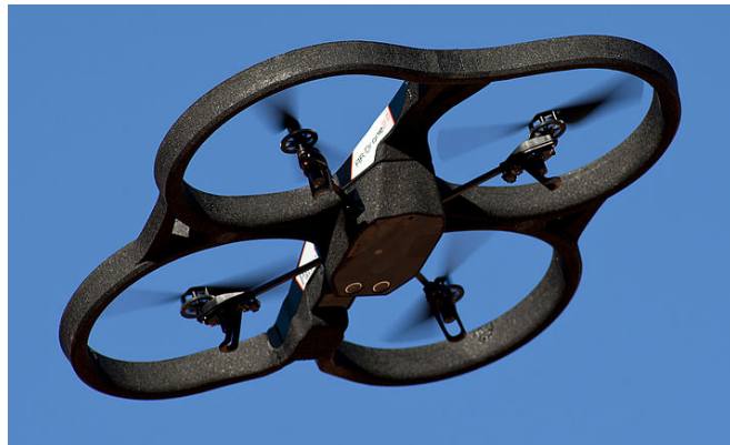
Figure 1.16 Parrot AR. Drone 2.0 equipped with its protective indoor hull.
