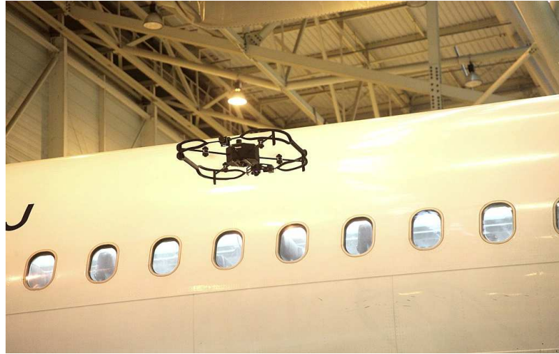
Figure 1.17 Donecle drone inspecting autonomously an AirFrance aircraft.
