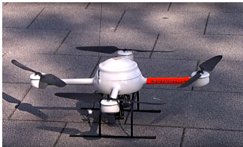
Figure 1.2 Microdrone MD4-200, Professional quadcopter with + Configuration.
