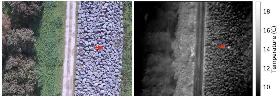
Figure 1.13 RGB (left) and TIR (right) images taken from the drone showing the same scene for a search and rescue scenario. The volunteer hiding in rocks is very difficult to discern in the RGB image but appears as a bright source in the TIR image [19].
