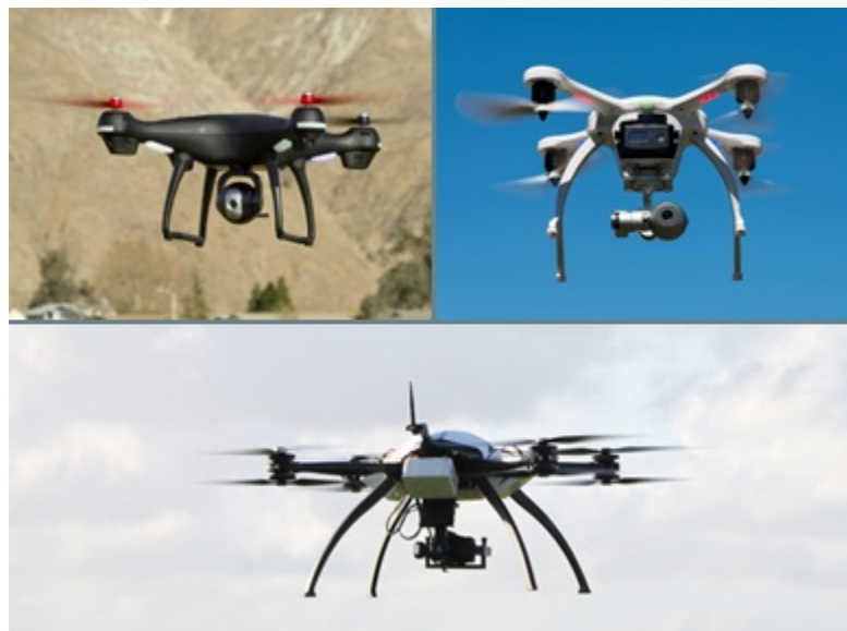
Figure 2.2 Propulsion configurations: tractor (top left), pusher (top right), and co-axial (bottom).
