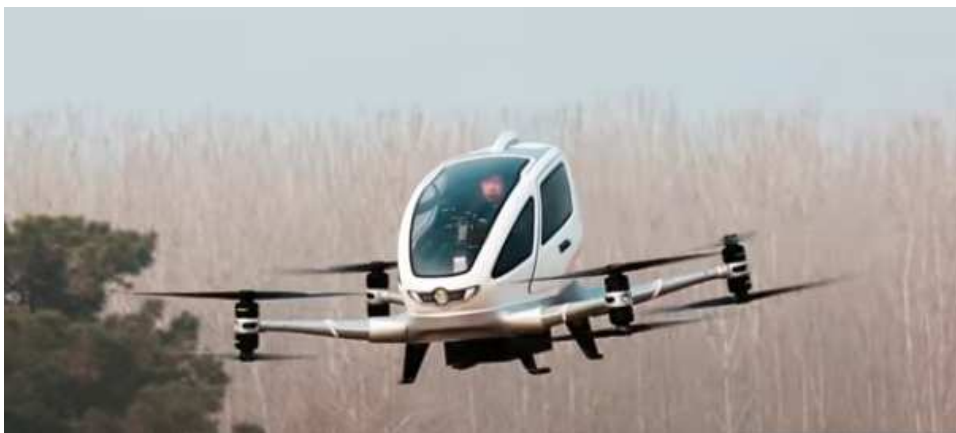
Figure 1.19 Ehang 184, autonomous manned quadcopter for air transport uses.
