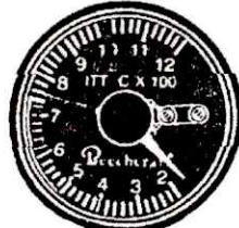
Interstage turbine temperature
