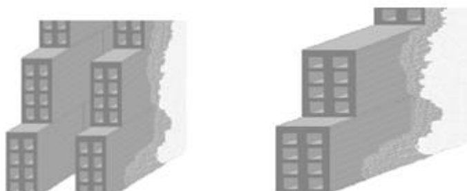
Figure 2. 9: Mur simple et double cloison
