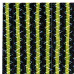
Figure 1.10 - Tissu hybride carbone - aramide
