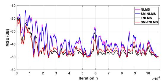
Figure.2.6. The Comparison of the initial convergence and the steady-state MSE. Input: speech signal with Car system of length L = 1024. SNR=50 dB.
