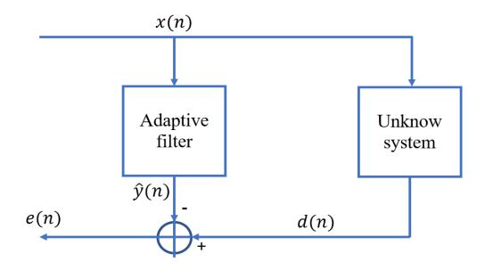
Figure 1. 4: The bloc diagram of system identification.
