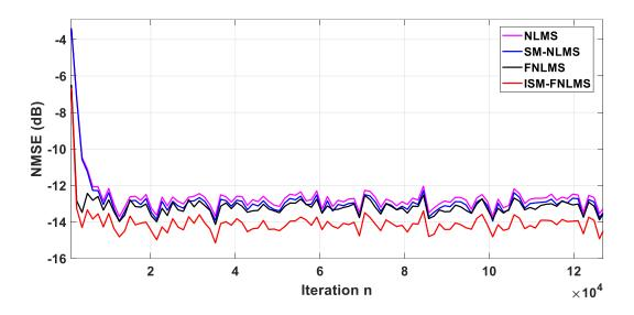
**Figure.2.12**. Comparison with noisy input: USASI signal with car system of length L = 256. Output noise: SNR=15 dB. Threshold  $\zeta = 0.1$ .  $\sigma_y^2 = 0.38$ .
