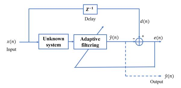
Figure 1. 6 : The bloc diagram of inverse modeling.
