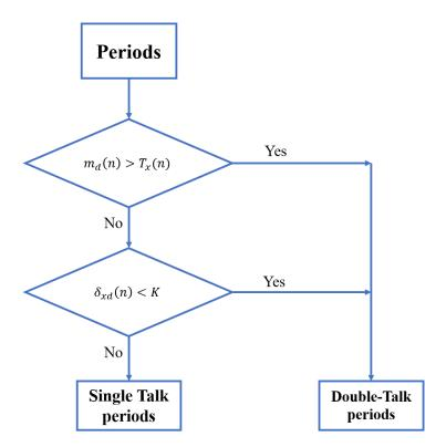
Figure.3.4. The flowchart of the DTD based on joint signal energy and cross-correlation estimation [59].
