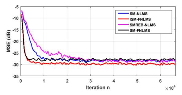
**Figure.2.22**. Comparison of SM algorithms with car system of length L = 256.Input USASI noise. Output noise: SNR=30dB. Threshold  $\zeta = 0.025$ .
