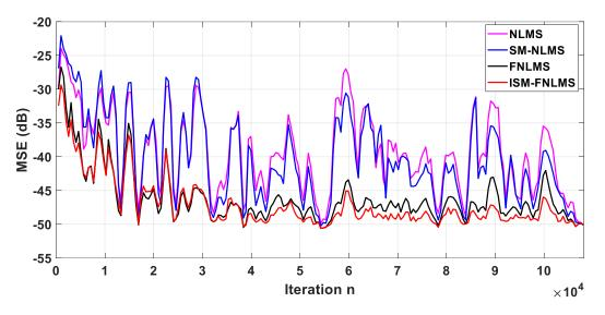
Figure.2.21. MSE evaluation Input: Speech signal with VCN system of length L = 1024. Output noise: SNR=50dB.
