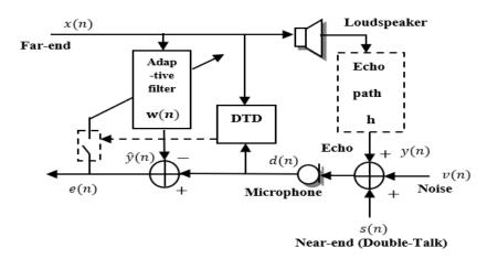
Figure.3.1. General structure of the AEC with DTD.
