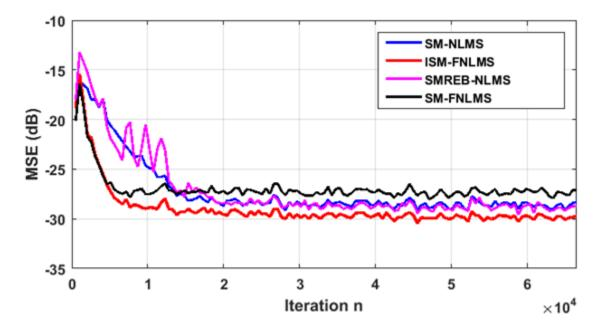
**Figure.2.23**. Comparison of SM algorithms with VCN system of length L = 1024.Input USASI noise. Output noise: SNR=30dB. Threshold  $\zeta = 0.025$ .
