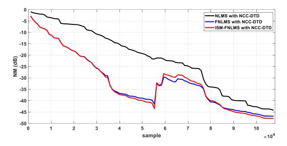
Figure.3.8. NM of ISM-FNLMS, FNLMS and NLMS with DTD in VCN system of L = 1024.
