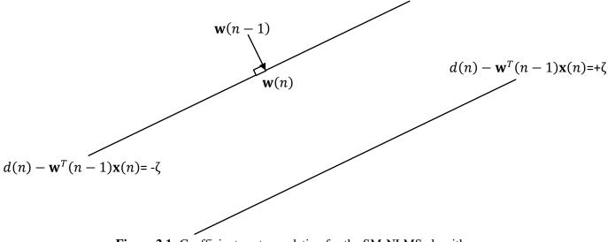
Figure 2.1: Coefficient vector updating for the SM-NLMS algorithm.
