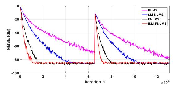
Figure.2.15. Comparison of the initial convergence and the re-convergence after an abrupt change in the impulse response of car system of length L = 256. Input: USASI noise. No output noise.
