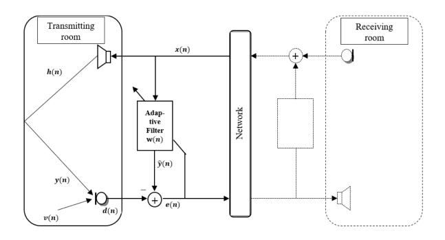
Figure.1.2. Basic AEC setup in a teleconferencing system.
