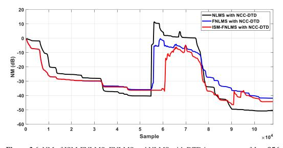
**Figure.3.6**. NM of ISM-FNLMS, FNLMS and NLMS with DTD in car system of L = 256. Figure 3.7 is the comparison of the output error waveforms for the three algorithms, on the DT segment, the output of the NLMS and FNLMS algorithms with DTD have an obvious distortion. In the other hand, the output of the ISM-FNLMS algorithm with DTD achieved the lowest distortion.
