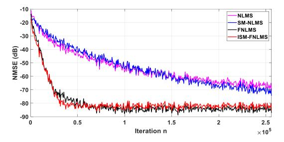
Figure.2.10. Comparison of the initial convergence and the SS-NMSE. Input: WGN-AR(20) signal with VCN system of length L = 1024. No output noise.
