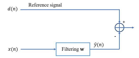
Figure 1. 8: Wiener filtering scheme.
