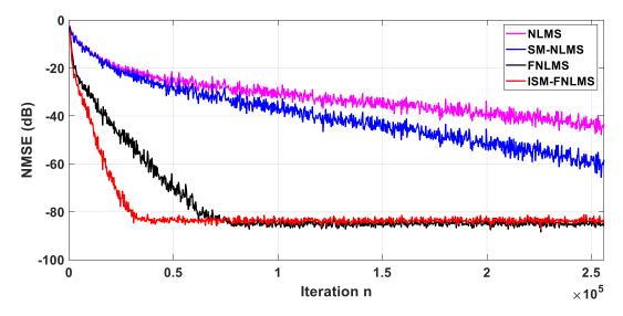
Figure.2.9. Comparison of the initial convergence and the SS-NMSE. Input: WGN-AR(20) signal with Car system of length L = 256. No output noise.
