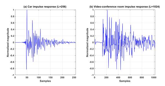
Figure.2.8. The used real acoustic impulse responses.
