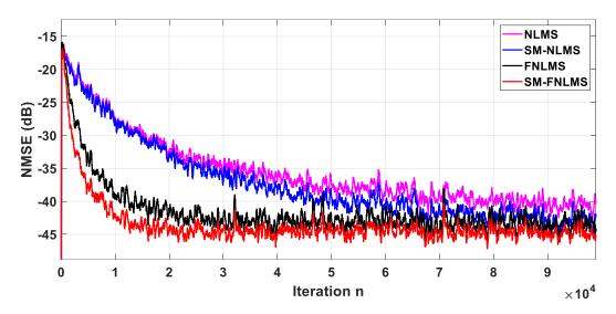
Figure.2.4. The Comparison of the initial convergence and the steady-state NMSE. Input: WGN-AR(20) signal with Car system of length L = 1024. SNR=50 dB.
