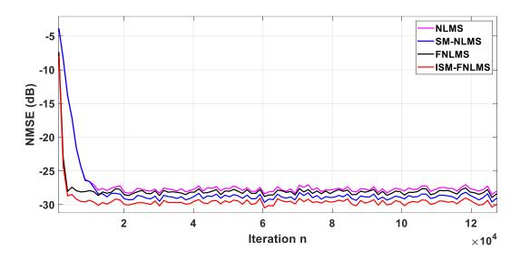
**Figure.2.13**. Comparison with noisy input: USASI signal with car system of length L = 256. Output noise: SNR=30 dB. Threshold  $\zeta = 0.025$ .  $\sigma_y^2 = 0.38$ .
