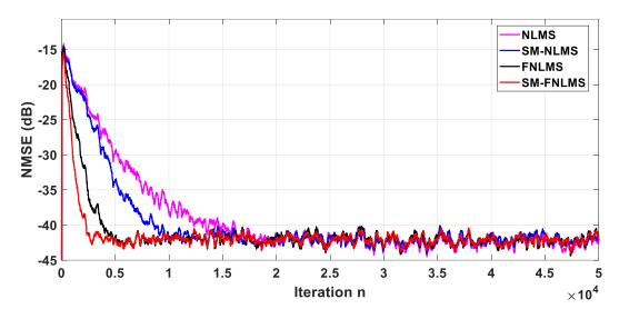
Figure.2.5. The Comparison of the initial convergence and the steady-state NMSE. Input: USASI signal with Car system of length L = 1024. SNR=50 dB.
