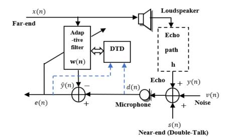
Figure.3.2. Basic structure of the AEC with DTD based on NCC.
