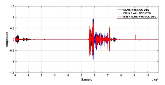
Figure.3.7. Output waveforms of ISM-FNLMS, FNLMS and NLMS with DTD in car system of L = 256.
