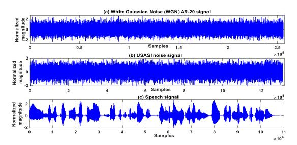
Figure.2.2. The used normalized input signals. (a) WGN AR-20 signal with a length of 256000 samples, (b) USASI noise signal with a length of 131072 samples, (c) Speech signal with a length of 108208 samples.
