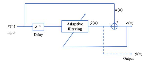
Figure 1. 5 : The bloc diagram of direct error prediction.
