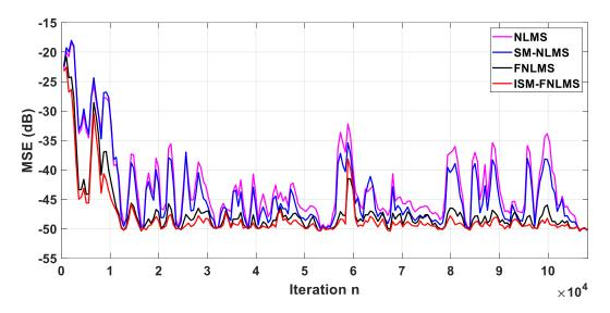
Figure.2.20. MSE evaluation Input: Speech signal with car system of length L = 256. Output noise: SNR=50dB.
