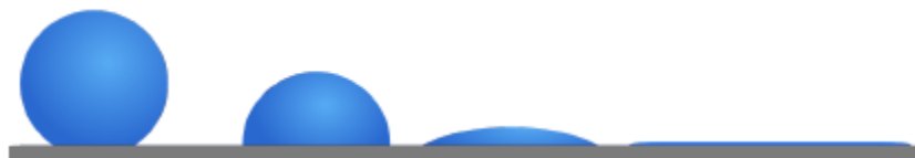
Figure 2-6: Figure of different wetting properties of different fluids with increasing wetting from left to right. [71]
