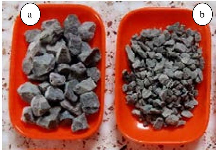
Figure 4.4: Gravier 8/15(a), Gravier 3/8(b).
