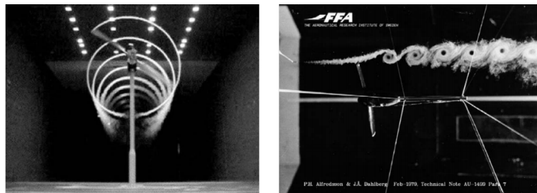
Figure 3.4: Visualization of the wake by the smoke in a wind tunnel
