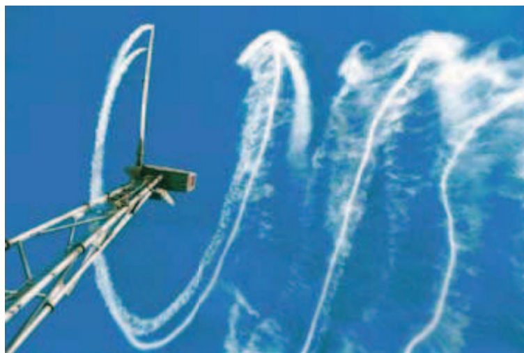
Figure 3.5: Wake structure downstream of a wind turbine, revealed by smoke; Risoe1997
