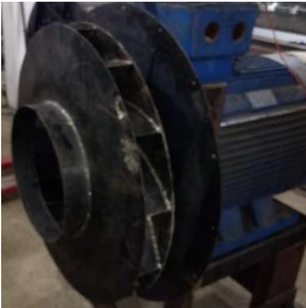
*Photo 5.1: Impeller attached to the electric motor*
