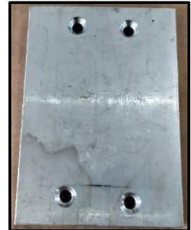
Figure 3. 28 : La plaque support de broche
