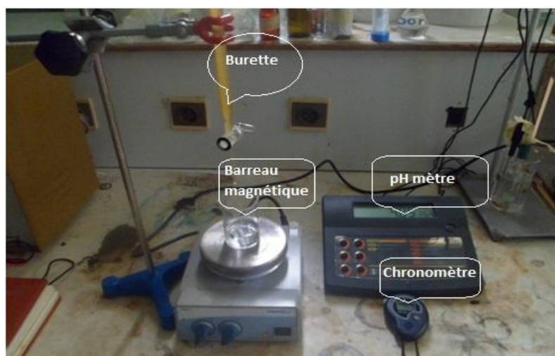
Figure III.6: Montage du profil neutralisation.
