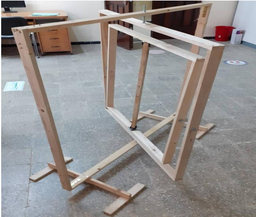
Figure (IV -18): Back view of the three frames test bench.
